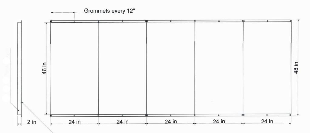
Encased in an 18-ounce vinyl coated nylon cover. The vinyl cover is fire- retardant, puncture and mildew resistant.
